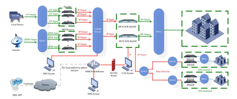
IP headend solution enable the cost reduction, more flexibility and easier management
